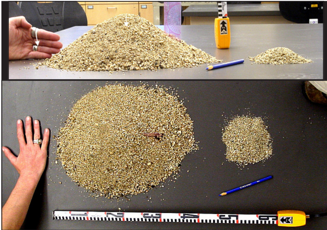
Figure 17: Bedload material collected on February 19, 2004. Left pile is 5260 g collected from Joshua Creek. Right pile is 710 grams collected from Garrapata Creek. Sampling time for both creeks was 20 minutes.
