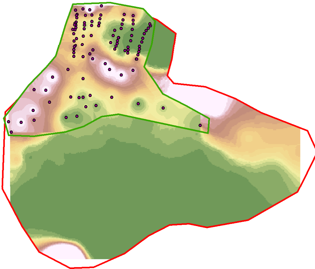
Figure 13: December 4, 2008 total station data point cloud and interpolated raster plotted on top of November 11, 2008 clipped raster. Both rasters were clipped using appropriate user-created mask. White corresponds to the higher elevations and dark green corresponds to the lower elevations. Color ramp used for each survey dataset is identical, providing the ability to qualitatively examine variability within the system.
